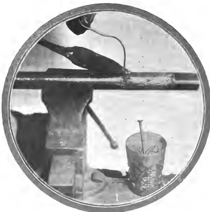
Fig. 1—Showing how the jackshaft may be tinned to increase its diameter so as to prevent leakage of lubricant
